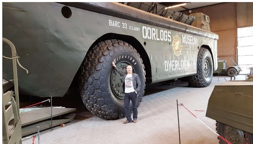
A BARC at a US military museum. The wheel is 9' diameter. From internet.
